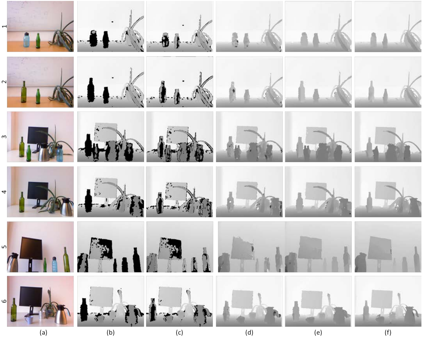
Fig. 6. Refined depth maps; (a) color images, (b) original depth images, (c) our cross modal stereo (CMS) results with Rank transform, (d) CMS + inpainting results, (e) CMS + MRF results, (f) our algorithm results.
