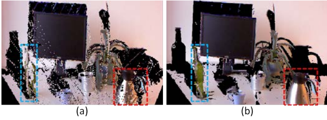
Fig. 7. 3D Point cloud reconstructions for; (a) cross-modal stereo [2] (b) our algorithm.
