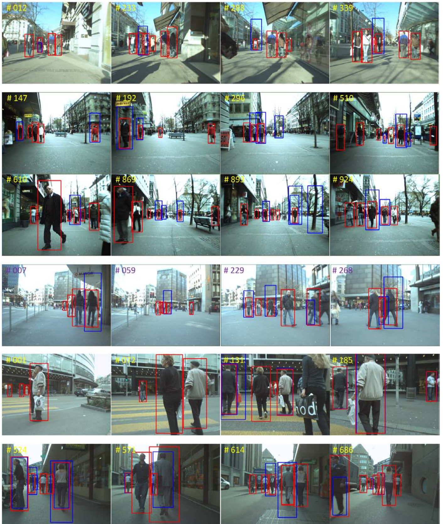
Fig. 3. Pedestrian tracks obtained using proposed ODPM (in red) and DPM (in blue) on the Sunny day , Bahnhof , Jelmoli , Crossing , and Linthescher videos from the ETH pedestrian data set. Figure best viewed in color.
