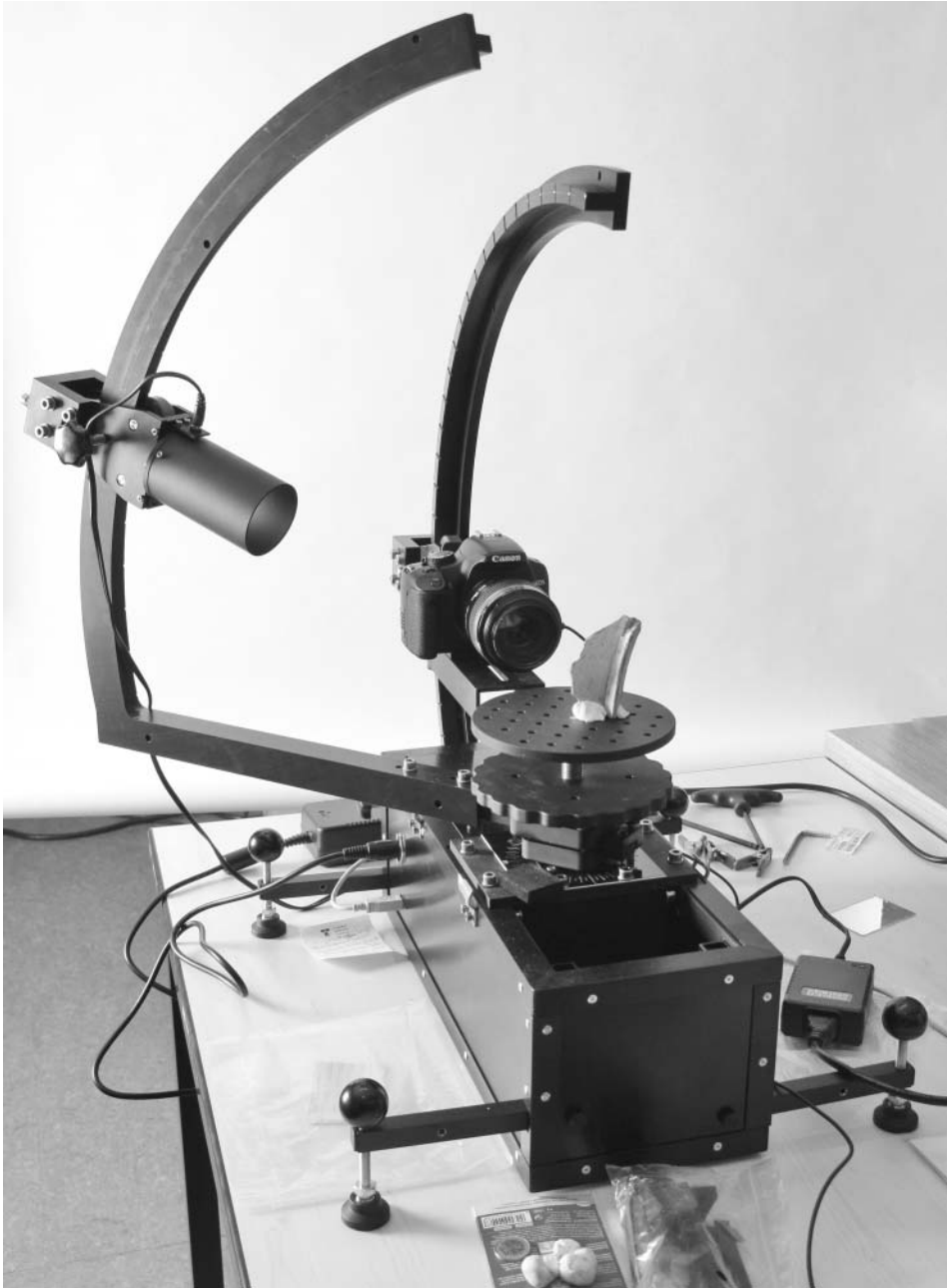
FIGURE 2 The acquisition device rotating a Roman potshard.
